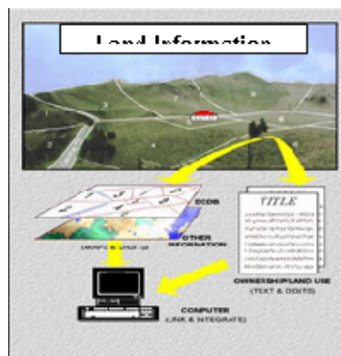
Fig.3: Components of a Land Information System (LIS)
